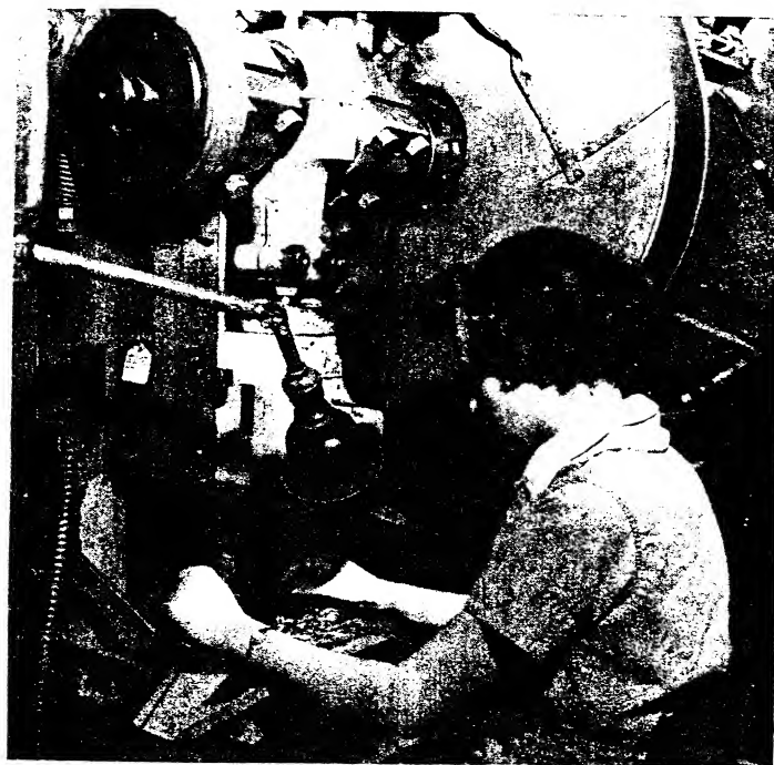
NO. 8—This 20-ton punch press raises the flat blank into the curved shape of a finished nib. The employee is Eileen Box.
